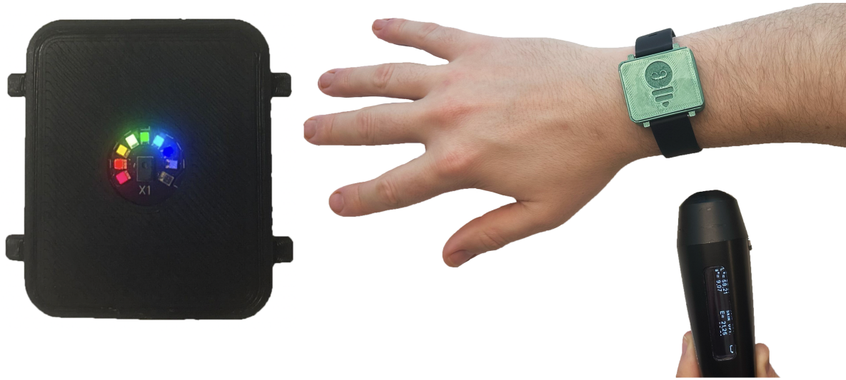
Fig. 1. DermaGlow is an advanced framework that utilizes wearable, multi-wavelength optical spectroscopy to deliver low-cost, continuous, and non-invasive measurements of melanin, erythema, and skin-color accurately across various skin tones and body locations.
